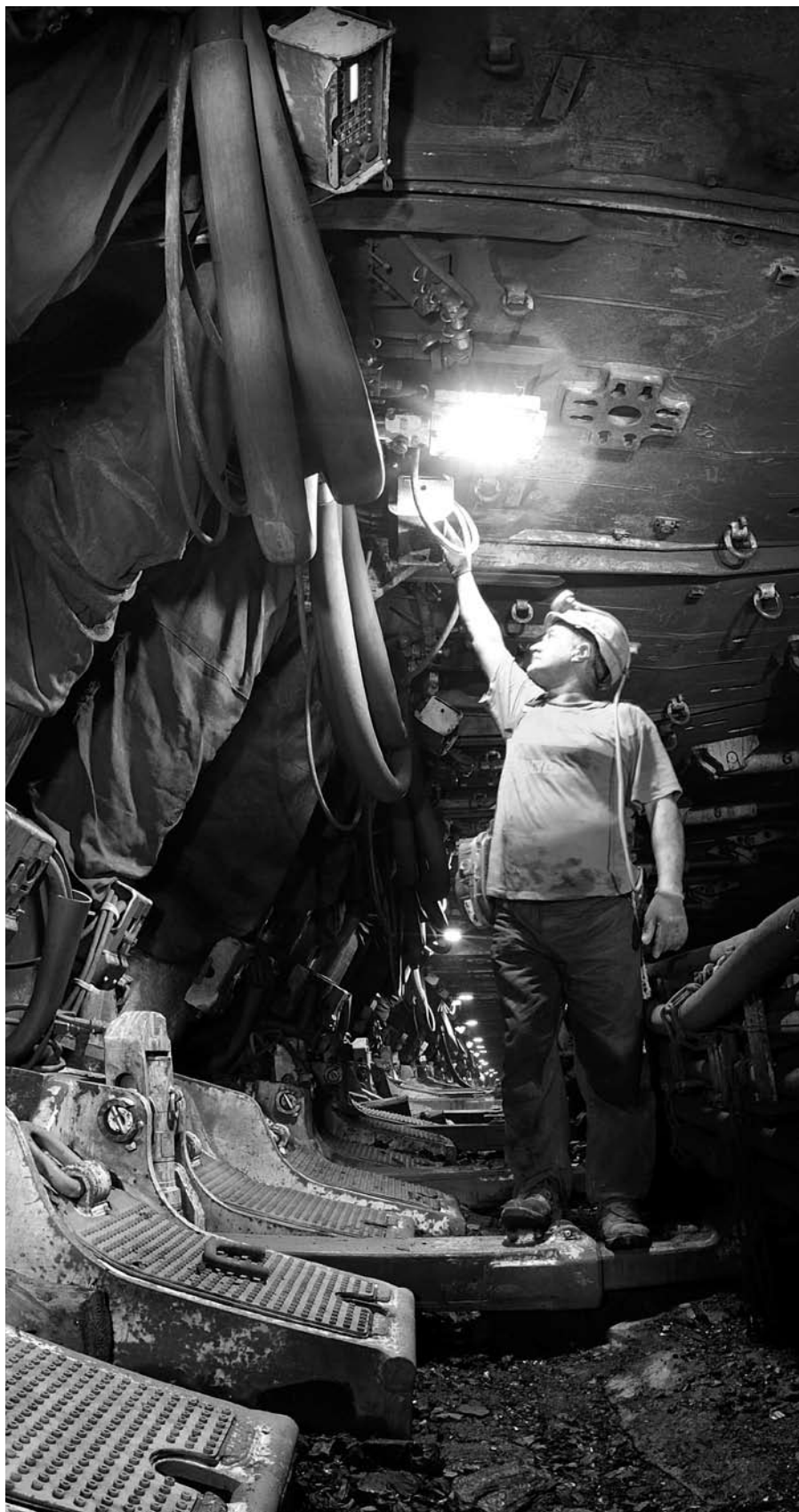
Mid-seam POP 2010 equipment set: shields
